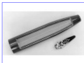
Cross-section of South African Mechem RO 122 PFHE warhead showing steel spheres cast in an epoxy resin sleeve around the explosive warhead filling; also visible is a cross-sectioned Fuchs Electronics BM21 radio proximity fuze
