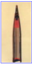
Warhead of NORINCO 122 mm Shrapnel rocket, also known as Rocket Steel Ball Shell, containing 4,100 steel balls
