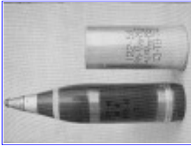
The 122 mm Illuminating projectile and cartridge case produced by NORINCO for the 122 mm Howitzer Type 54
