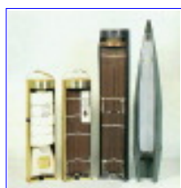
Cross-sectioned 152 mm FRAG-HE 3OF45 projectile on right with, from left: Reduced charge; Full charge; and Long Range charge (1998)
