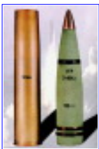
Iranian 130 mm Smoke projectile and cartridge case (2000)
