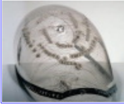
The effect of a single 35 × 228 mm AHEAD projectile on an aircraft cockpit canopy (1998)
