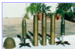
A selection of 85 mm rounds, from left: HEAT-FS BK-367; HVAP-T BR-365PK; HEAT-FS BK-2 (1999)
